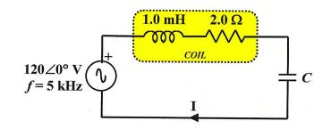
(a) [15 points] Determine the value of capacitance C that will cause the system to be in resonance.
