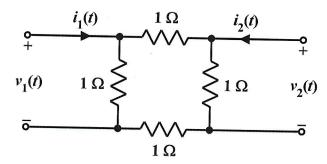
(a) [16 points] Determine the hybrid-parameter (*h*-parameter) representation and express it in the standard matrix form.
